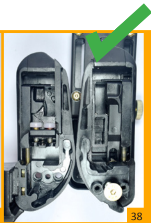
The height of the box on side B has been correctly matched to the height of side A.
